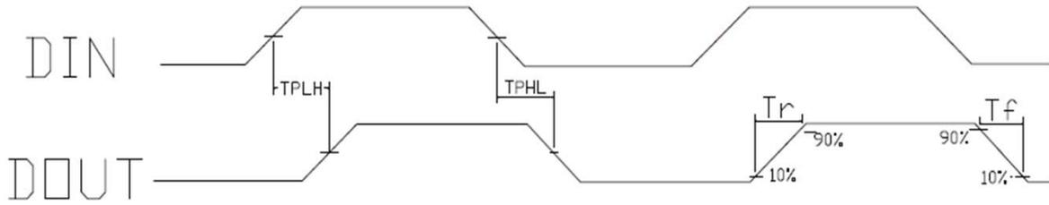
10. The data transmission time (T<sub>H</sub>+T<sub>L</sub>=1.25μs±600ns):
