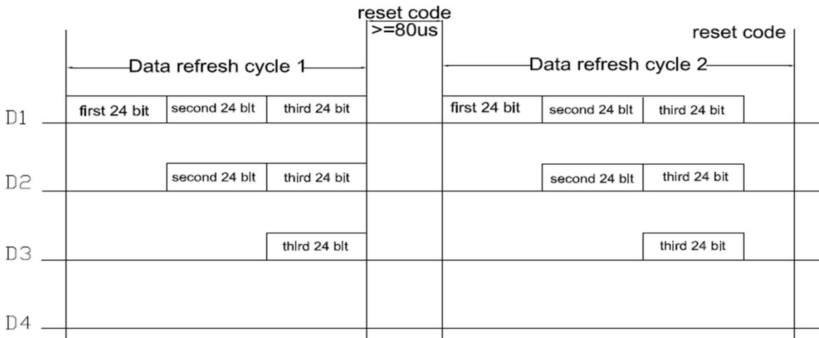
Note: the D1 sends data for MCU, D2, D3, D4 for data forwarding automatic shaping cascade circuit.
