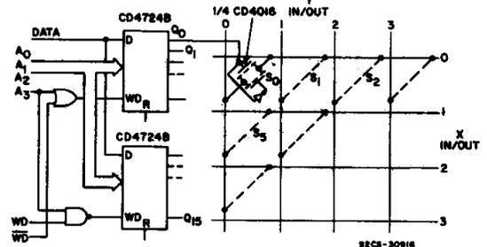
Fig. 16— Multiple selection decoding — 4 x 4 crosspoint switch.
