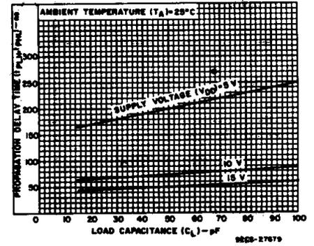
Fig. 8 - Typical propagation delay time (data to Q<sub>n</sub>) vs. load capacitance.
