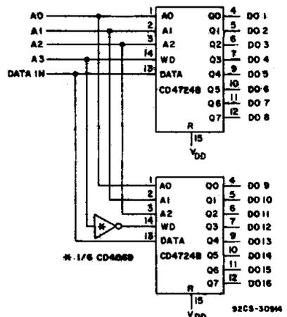
Fig. 14— 1 of 16 decoder/demultiplexer.
