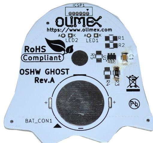
Then you need for find three resistors in paper tape, they are marked 121 = 120 or 120 Ohms! These must be soldered to R1, R2, and R4 locations:
