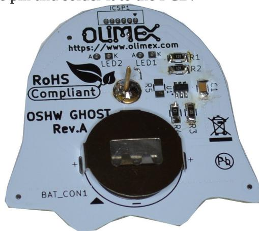
We are almost done! Now put the LEDs on their places, but note that they have POLARITY so you have to put them with the shorter leg inside the square pad (marked as K) and longer led in the circle pad (marked as A).
