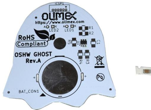
You must peel the transparent tape and take off the capacitor then to solder it to C1 pads on the board like on this picture.
