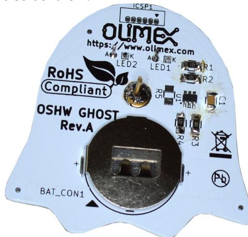
Now is time to attach the battery, again be careful as battery has polarity the + must be pointing UP as on this picture:
