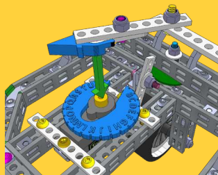
F : Put the Servo Arm with Index Arrow back on the servo matching the "O" mark on the disc.
